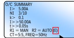
The letter in brackets refers to whether Relay 2 has been set to trigger at the start or end of the time out period.
